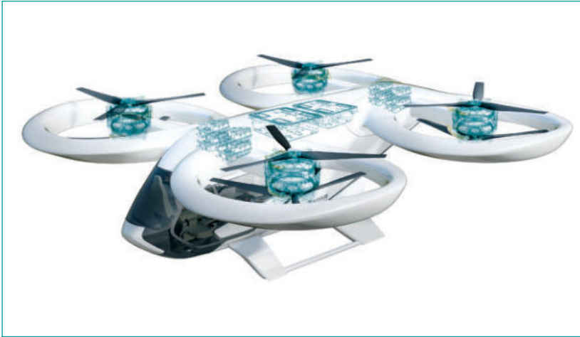
Air taxi CityAirbus: the demonstrator of Airbus' four-seat e-VTOL is being jointly developed with Siemens. It will be powered by eight distributed motors. ■
