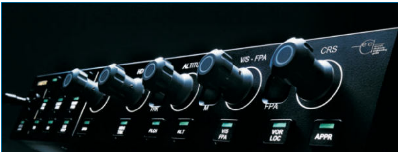
Mode Control Panel - Allows crew to select which parts of the aircraft's flight is automatically controlled ■
