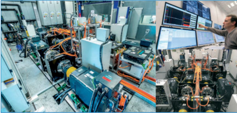
Airbus E-Aircraft Systems Test Lab at Taufkirchen for system integration testing of CityAirbus electric propulsion system developed in collaboration with Siemens AG. Testing of the full system on ground aims to verify the electric propulsion system functionality and performance considering its electric and mechanical dynamic sub-systems interactions at mission envelope. Therefore the electric propulsion system under test consist of the electrical power unit (8x120kW motors), 800VDC power distribution units, (4x30kWh) Li-Ion battery stacks and the air vehicle flight control system. ■
