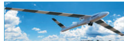
Fig. 4: Unmanned demonstrator for highly flexible wing concepts (EC H2020 Project FLEXOP) ■
