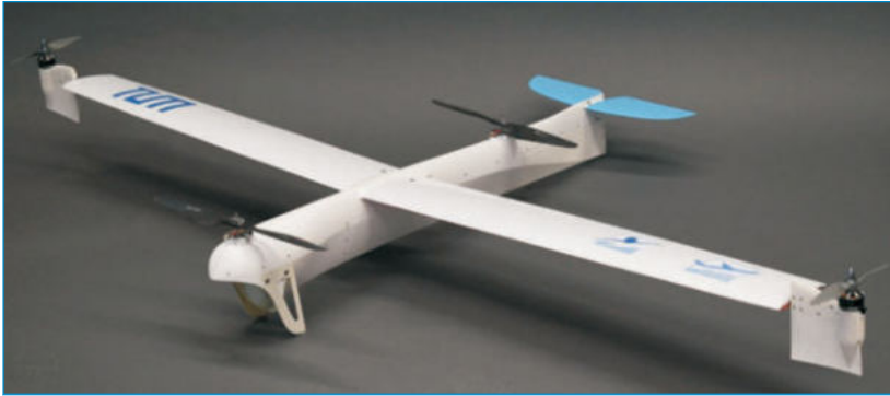
Fig. 2: Transition-UAV: high efficiency in cruise flight while providing vertical take-off and landing capabilities ■
